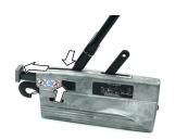
Fig. 3: Release the "Jockey" cable winch
